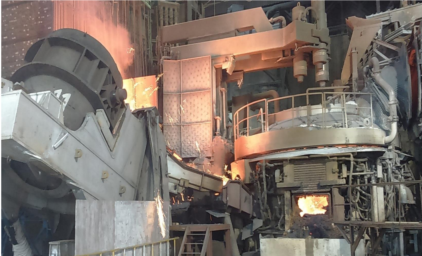
Tenova FMF ® furnace melting hot metal and scrap to produce steel
