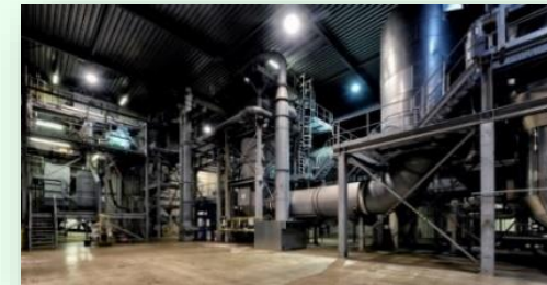
TorrCoal / Perpetual Next Rotary drum technology (small size feedstock)
